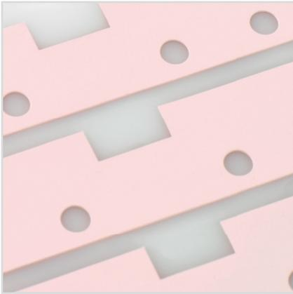
Keratherm 86/60 offers outstanding thermal conductivity, which is achieved by a specially filled silicone elastomer. The excellent electrical insulation properties are thereby retained. On request, these films can also be supplied with fibre glass reinforcement and with or without adhesive coating. The excellent thermal resistance of this film enables the optimum heat transfer to the heat sink.
